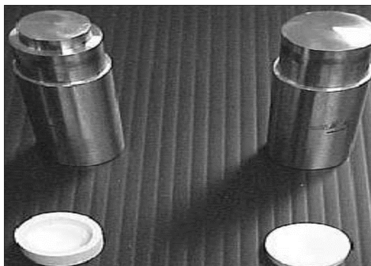
Fig 5: A photo showing the tooling used to illustrate Proof-of-Concept, as well as a cup and a completed dose form
