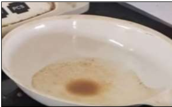
Fig 4: Determination percentage solid content of shampoo
